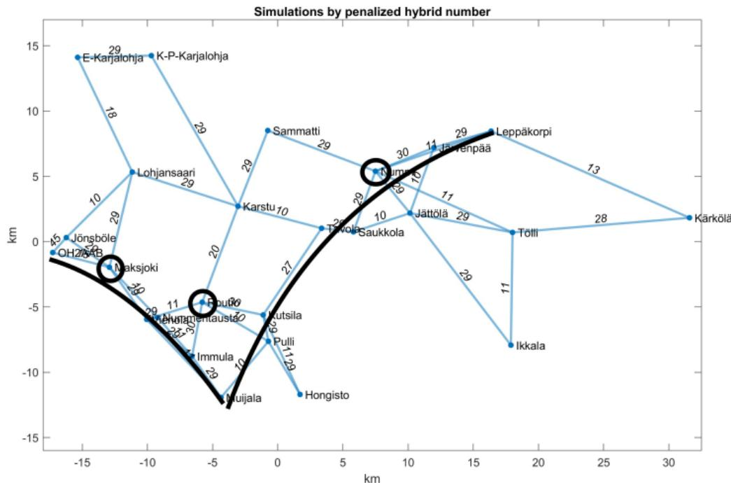
The proposed backbone radio network for Lohja area. Particularly important terrain corridors and the central points at Maksjoki, Routio and Nummi are shown by thick black line.
