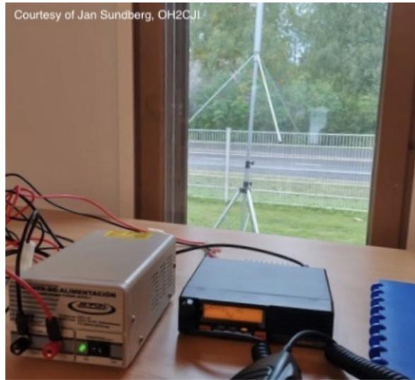
Both hand-held radiophones (TX power  $\leq$  5W) and tabletop base stations (TX power  $\approx$  25W as in picture) are used.
