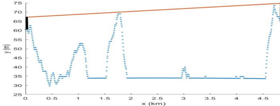
Mast number is the minimum total height of masts required for a line-of-sight connection between the endpoints.
