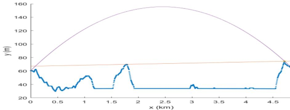
The curvature number  $\kappa$  is the angle of the circular arc per length  $L$ , where  $L$  is the distance of endpoints.
