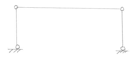
The above unstable truss is a mechanism. Another form of instability is a  $rigid\ body\ motion$
