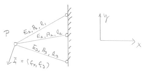
We have two equilibrium equations, but three unknowns, i.e. the forces in the bars. That is, the structure is statically indeterminate. In order to solve the problem, the elongations of the bars have to be taken into a account.
