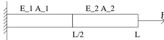
built of two different materials having different cross sections. As in previous problem, write down the three formulations (M), (V), and (D).
