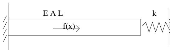
where  $f(x)$  is a distributed load and  $k$  is the spring constant. Write down the energy expression (M), principle of virtual work (V), and boundary value problem (D) for this problem.
