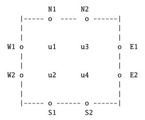
The solution of Laplace's equation models f.eg. the steady state temperature inside a metal plate whose boundary temperatures are held at the given temperature values. Replacing the  $2^{nd}$  derivatives by their difference approximations leads to the simple rule:
